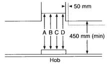
A: Built-in Electric Hob: 650mm minimum clearance
